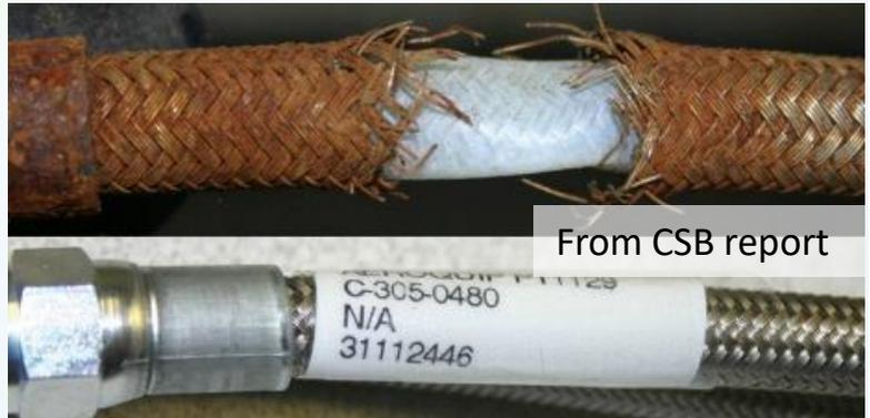
Under the label, the hose braiding corroded. The weak hose ruptured, spraying a nearby operator with Phosgene.
